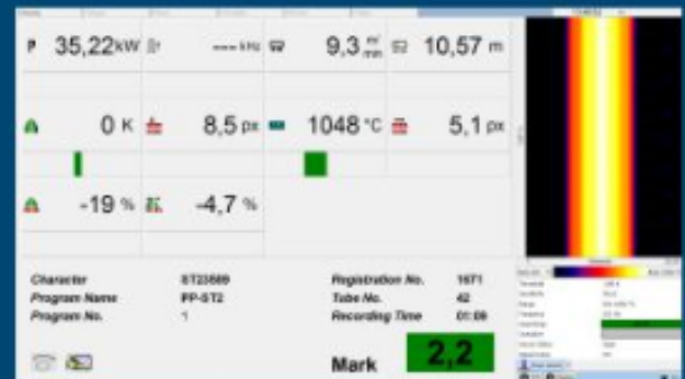
GUI during welding with automated seam evaluation
