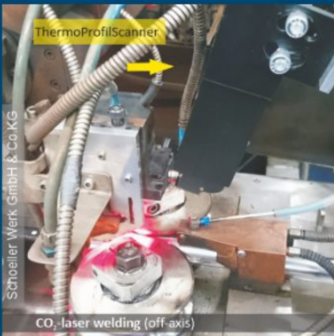
CO 2 -laser welding with disturbances of the process gas detected in the thermal field
